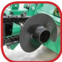
Auger clears dirt while trenching
