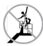
Do not sit, stand, or climb on the platform guard rails. Maintain a firm footing on the platform floor at all times.
