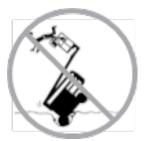
Use extreme care and slow speeds while driving the machine in the stowed position across uneven terrain, debris, unstable or slippery surfaces and near holes and drop-offs.
