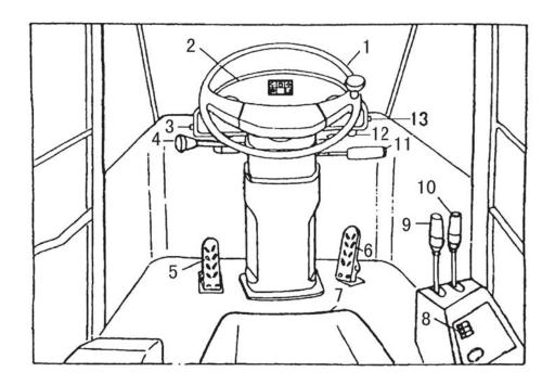
Steering wheel 2.Panel 4.Gearshift lever 5.Brake Pedal Steering
