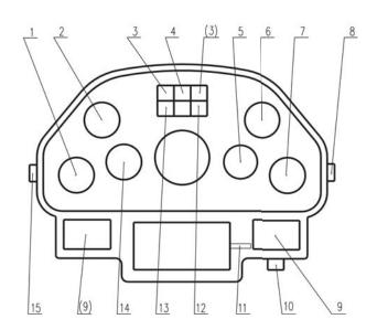
1. Engine Coolant Temperature Gauge
