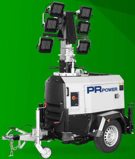
The PR-ECO LED Mobile Lighting Tower units utilise highly efficient LED lamps mounted atop an 7.8m vertical, hydraulic mast with a 48vDC extra low voltage lighting system and the Automatic Mast Operating Safety System (AMOSS) for added safety and environmental sustainability.
