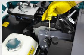
2. Check engine oil level and top up if necessary.
