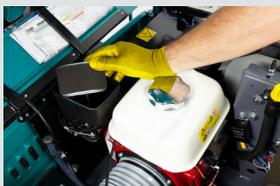
1. Clean the engine air intake filter.
