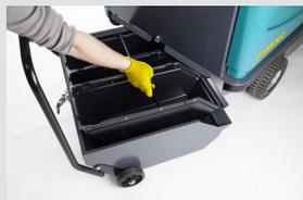
4. Remove the hopper and empty out the debris that has been collected.
