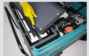
4. Check that the gaskets which seal the hopper are intact and in good condition.
