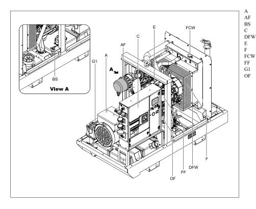
AAlternatorAFAir filterBSBattery switchCCubicleDFWDrain flexible cooling waterEEngineFFanFCWFiller cap cooling waterFFFuel filterG1BatteryOFOil filter
