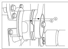
5. Measure 21 mm (0.83 inch) from (A) and put a mark (B) on the tensioner mounting base.
