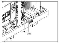
EFTExternal fuel tank feed connectionEFRExternal fuel tank return connection
