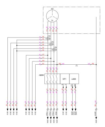
(\*) To remove this connection if IT-Relay is assembled
