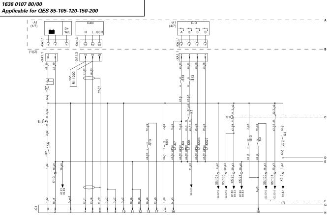
(\*) Terminals X5:102-103 must be bridged if the External Emergency Stop isn't mounted
