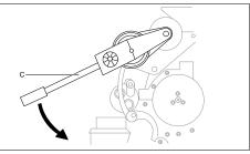
7. Rotate the swing arm using a torque wrench until marks (A and B) are aligned.
